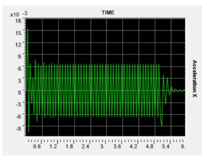
Figure 6 X-direction acceleration of portal structure Source: Data in Research,2020.
